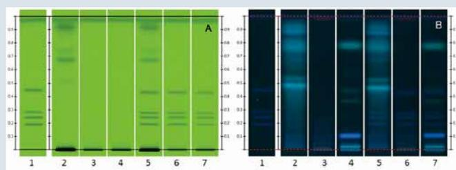
Chromatogram under (A) UV 254 nm and (B) UV 366 nm, track 1: sildenafil, propoxyphenyl hydroxyhomosildenafil, homosildenafil, hydroxyhomosildenafil with increasing  $hR_F$ ; tracks 2–4: plants extracts; tracks 5–7: spiked plant extracts
