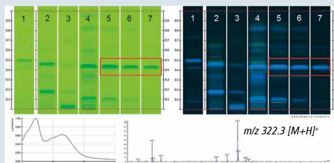
In-process control of the LSP: Chromatograms under UV 254 nm and UV 366 nm show the sequence of the synthesis and the purification steps (track 1: LSD as reference, 2: digest of the lysergic acid from ergotamine, 3: purified lysergic acid (starting material for the chemical synthesis), 4: crude synthesis product (LSP and side products), 5, 6: column purification steps, 7: finished product as well as the UV spectra and the mass spectra of the eluted LSP zone at  $m/z$  322.3  $[M+H]^+$
