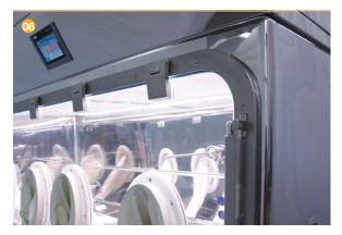
Inflatable sealing safety glass fitted with sleeved flanges and sensors for monitoring safe window closure. A gas spring is used for easy opening.
