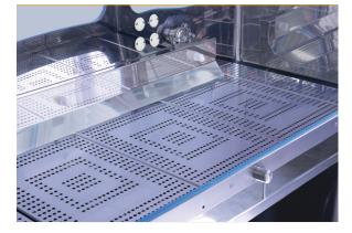
The worktop is equipped with 6 perforated grates. The grates can be fitted with a device for sterility testing.
