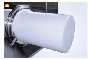
Option to integrate an RTP alpha port and beta container for sterile transfer of materials. Chamber's right wall is prepared for integration of the equipment.
